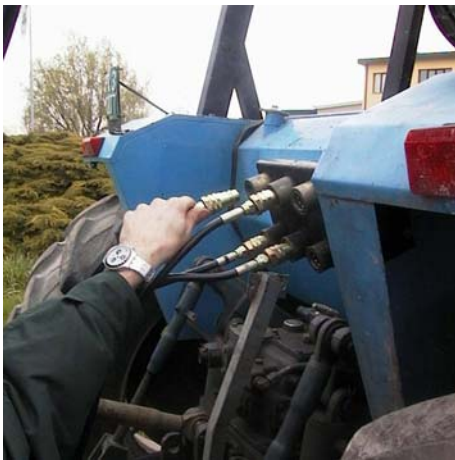
Tractor coupling for homologated Towed machines in work position (not suitable for road use).
